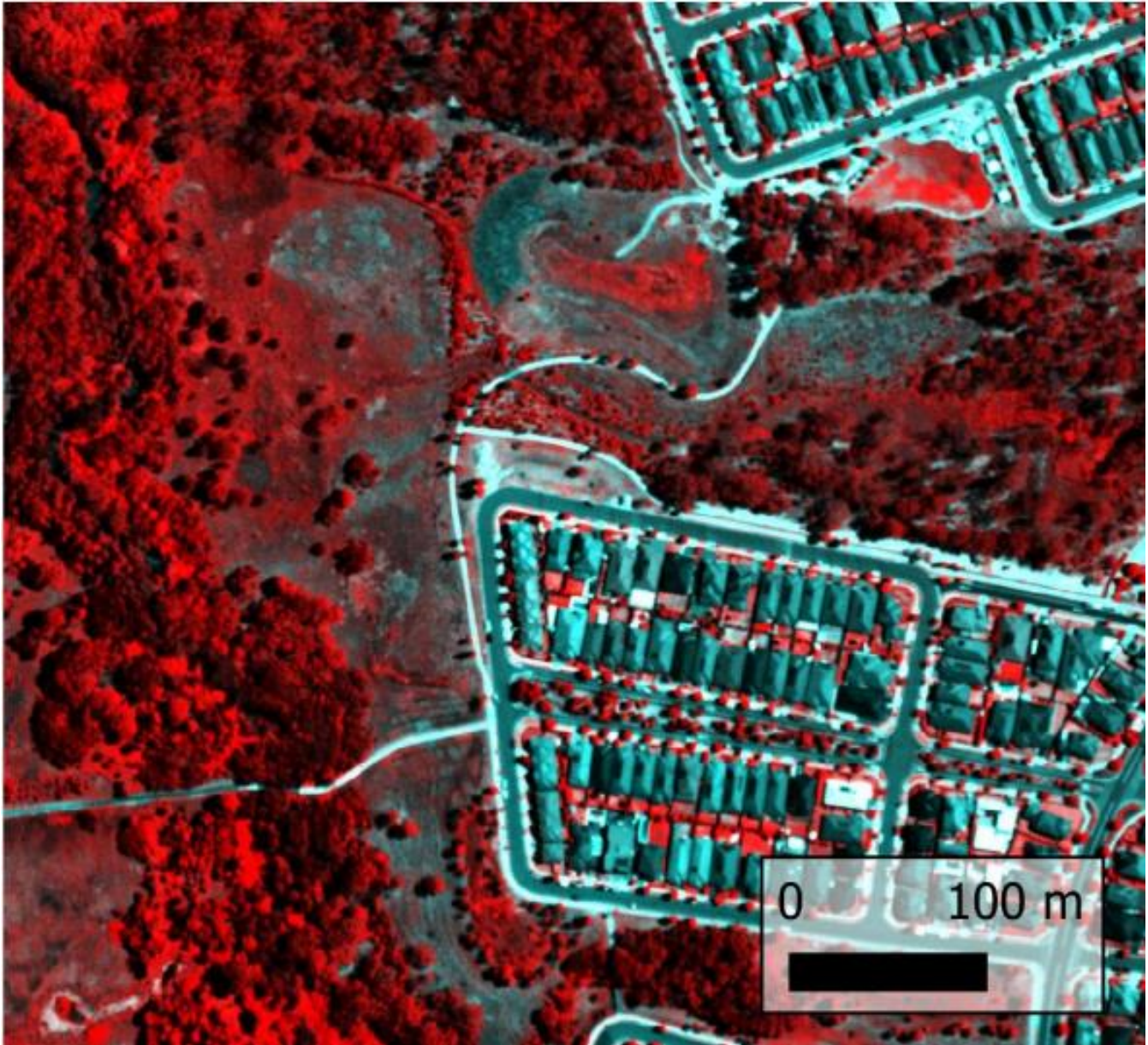
Figure 3: False Colour Composite (FCC) showing vegetation in red, derived from the 7-band multispectral imagery
