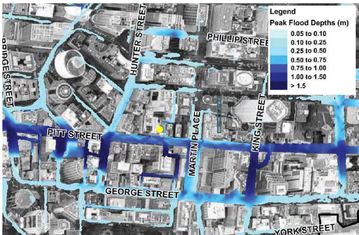
Figure 3 Probable Maximum Flood Depth (Source: BMT WBM., 2014)
