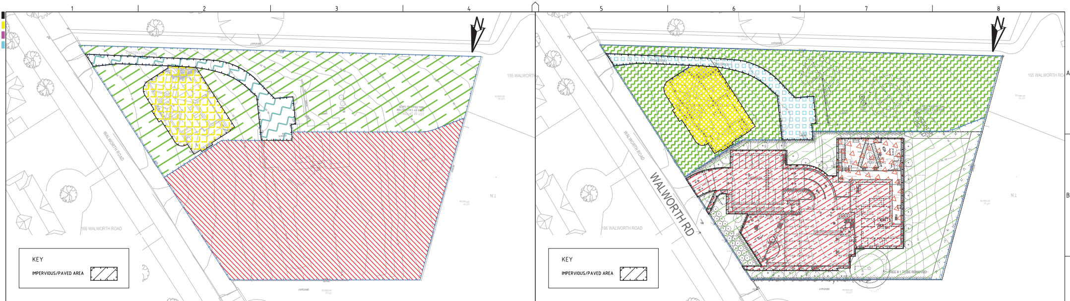
PRE-DEVELOPMENT OSD CATCHMENT PLAN SCALE 1500
