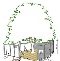
1. CHAIN WIRE MESH PANELS WITH SHADE CLOTH (IF REQUIRED) ATTACHED, HELD IN PLACE WITH CONCRETE FEET
