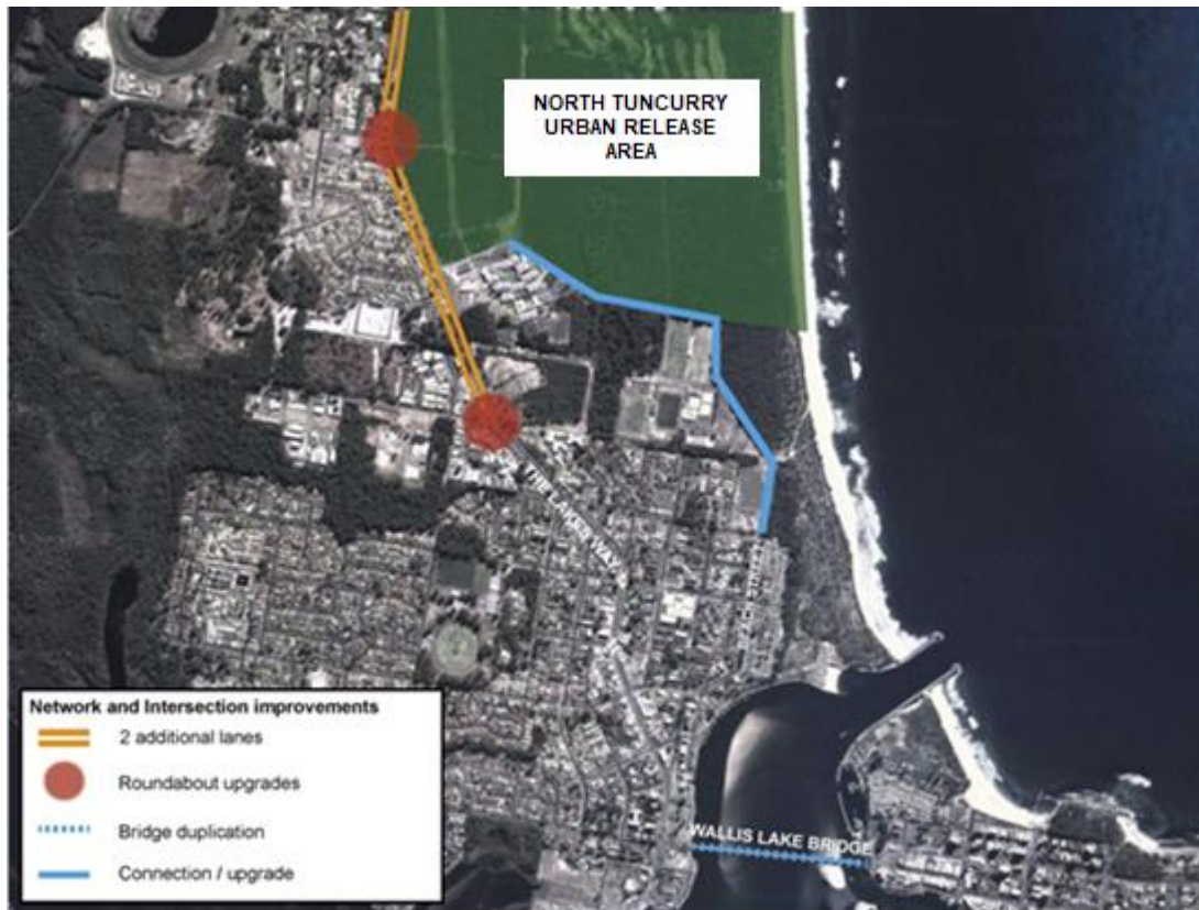
Figure 15 Road network and intersection improvements identified in the S94 Plan (for Tuncurry)
