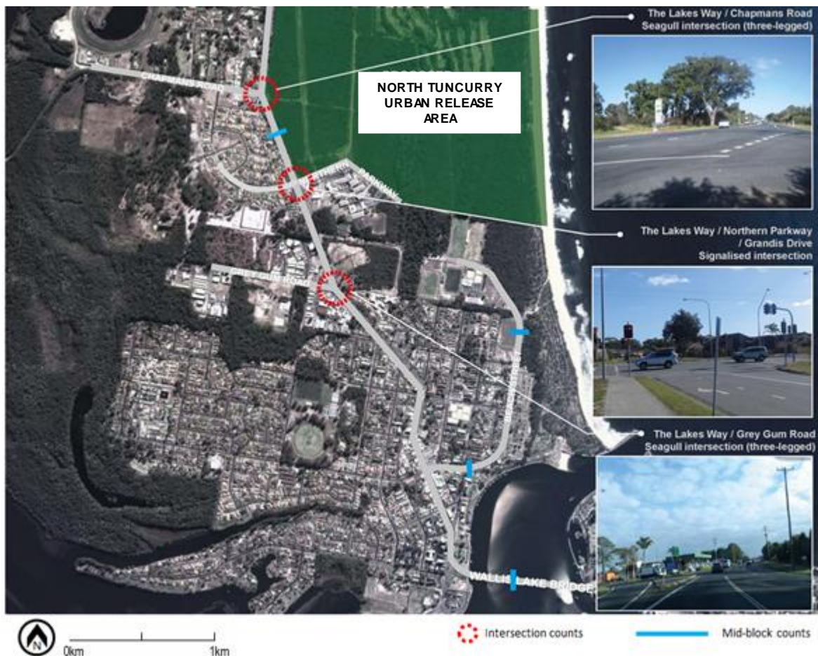
Figure 11 Traffic count survey locations
