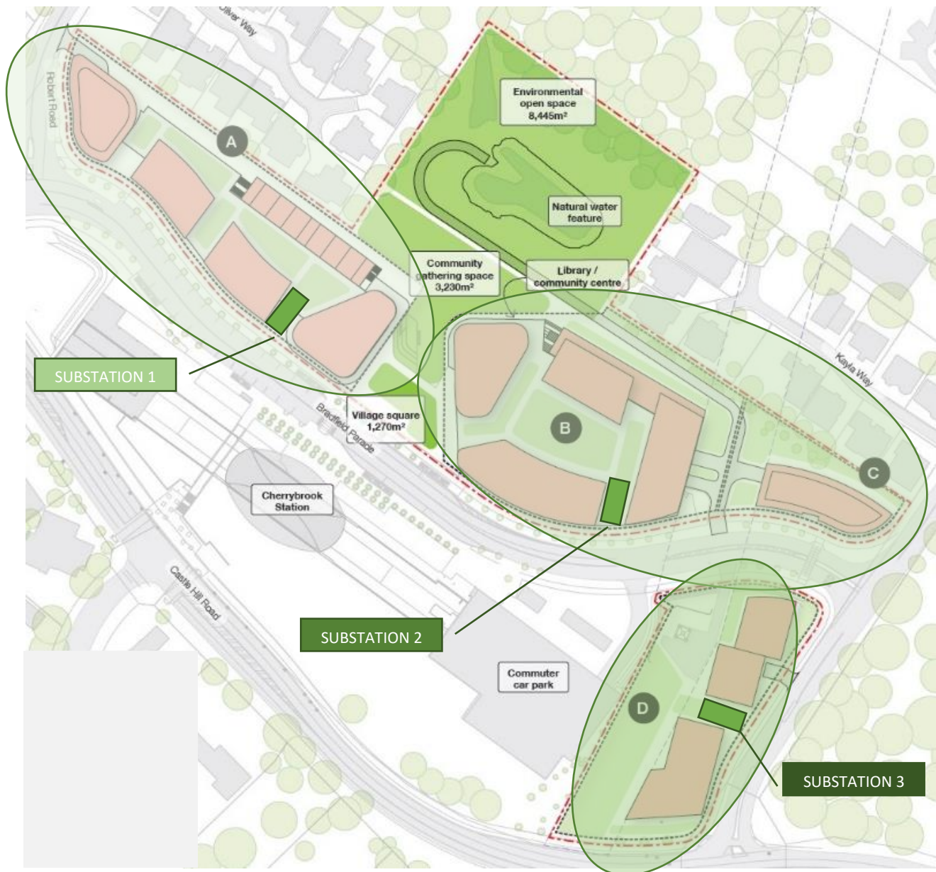
Figure 6 – Potential 11kV/400V substation locations and servicing options for the SSP Site based on the reference scheme
