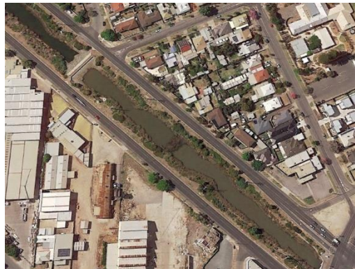
A section of Port Road, City of Charles Sturt, SA, in 2008 (left) and 2018 (right) showing the outcome of part of a large-scale water retention and storage Aquifer Recharge project which converted a cement drainage line and grassy swale into a thriving and biodiversity rich wetland whilst also managing stormwater, minimising flooding, and cooling the local environment (images from Google Earth).
