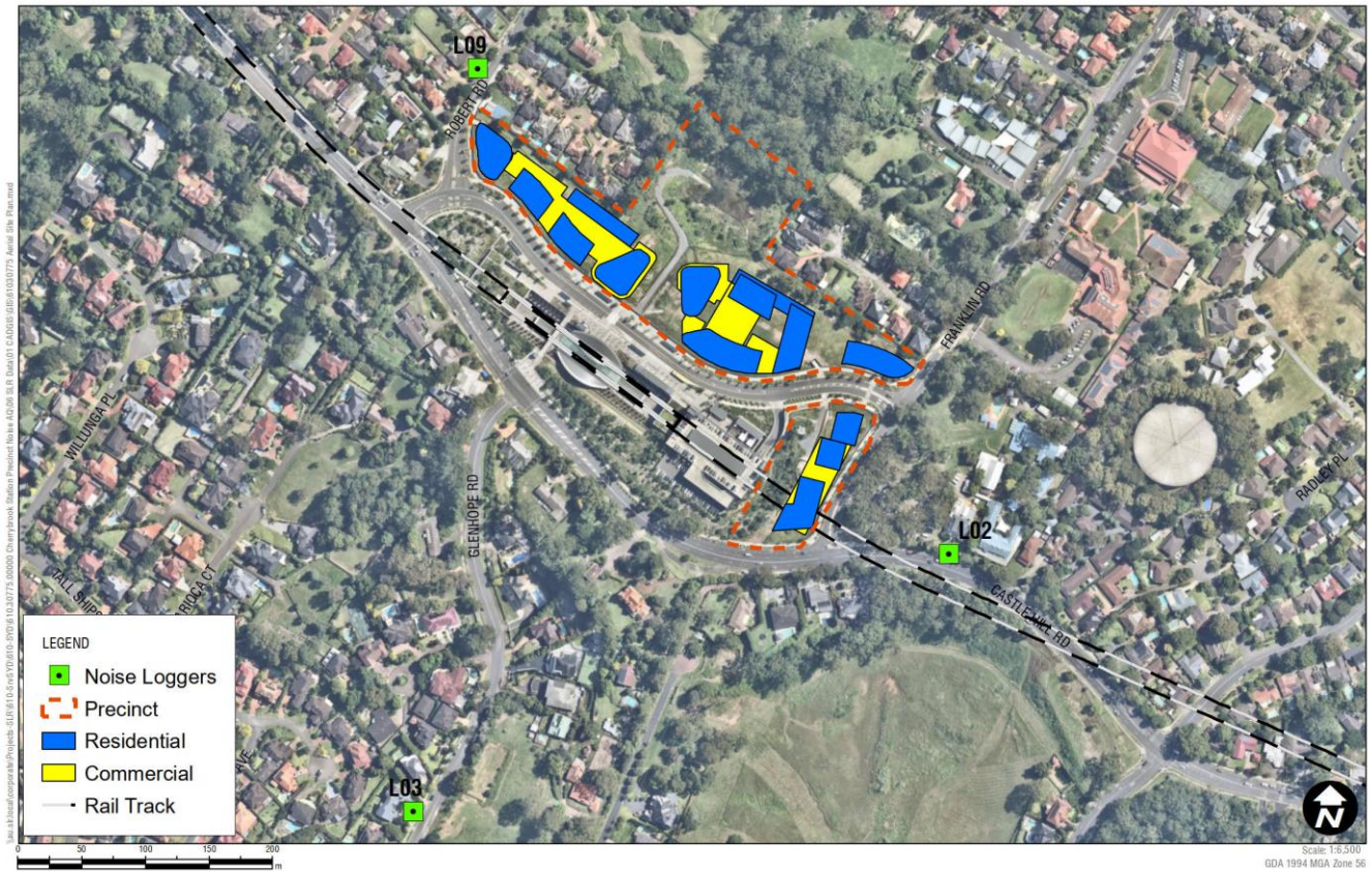
Figure 3 Site Plan and Noise Monitoring Locations
