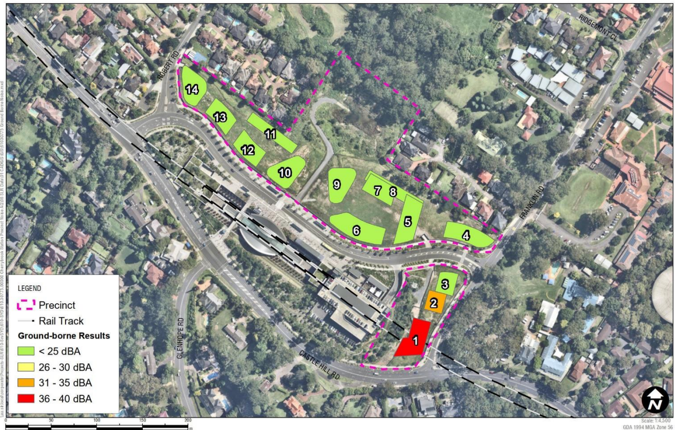
Figure 6 Predicted Ground-borne Noise Levels
