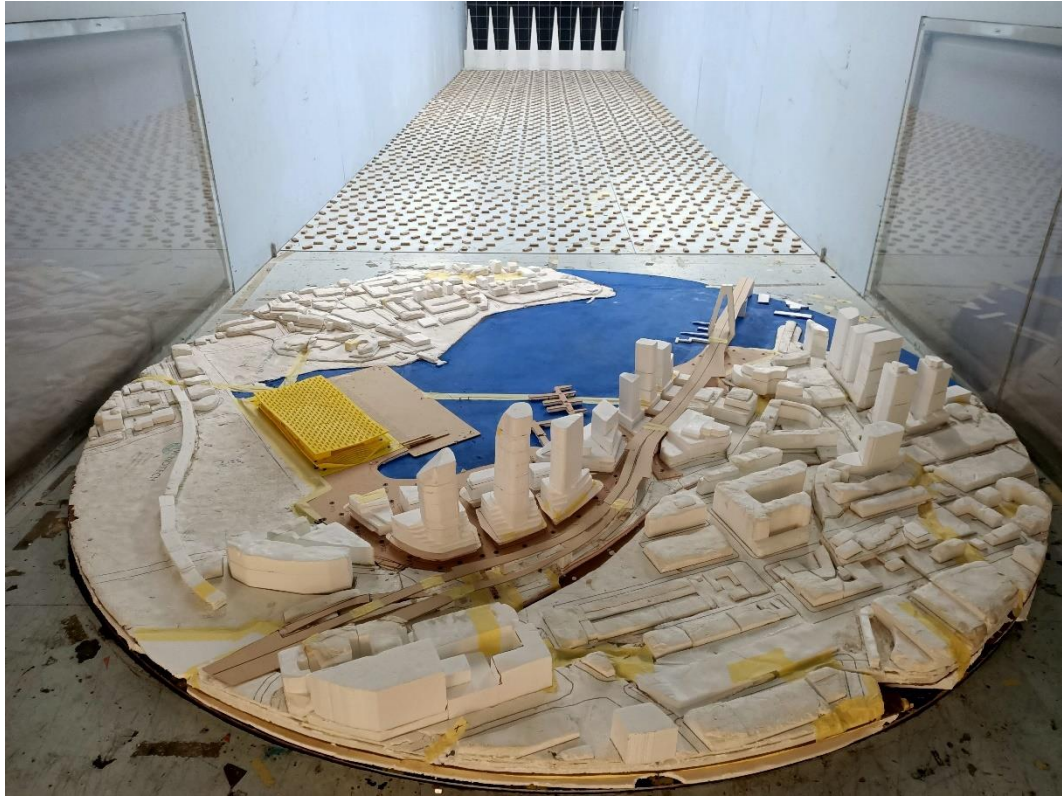
Figure 1b: Photograph of the Proposed Wind Tunnel Model (view from the east)
