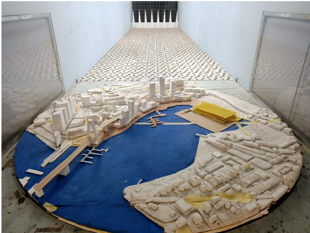
Figure 1d: Photograph of the Proposed Wind Tunnel Model (view from the west)
