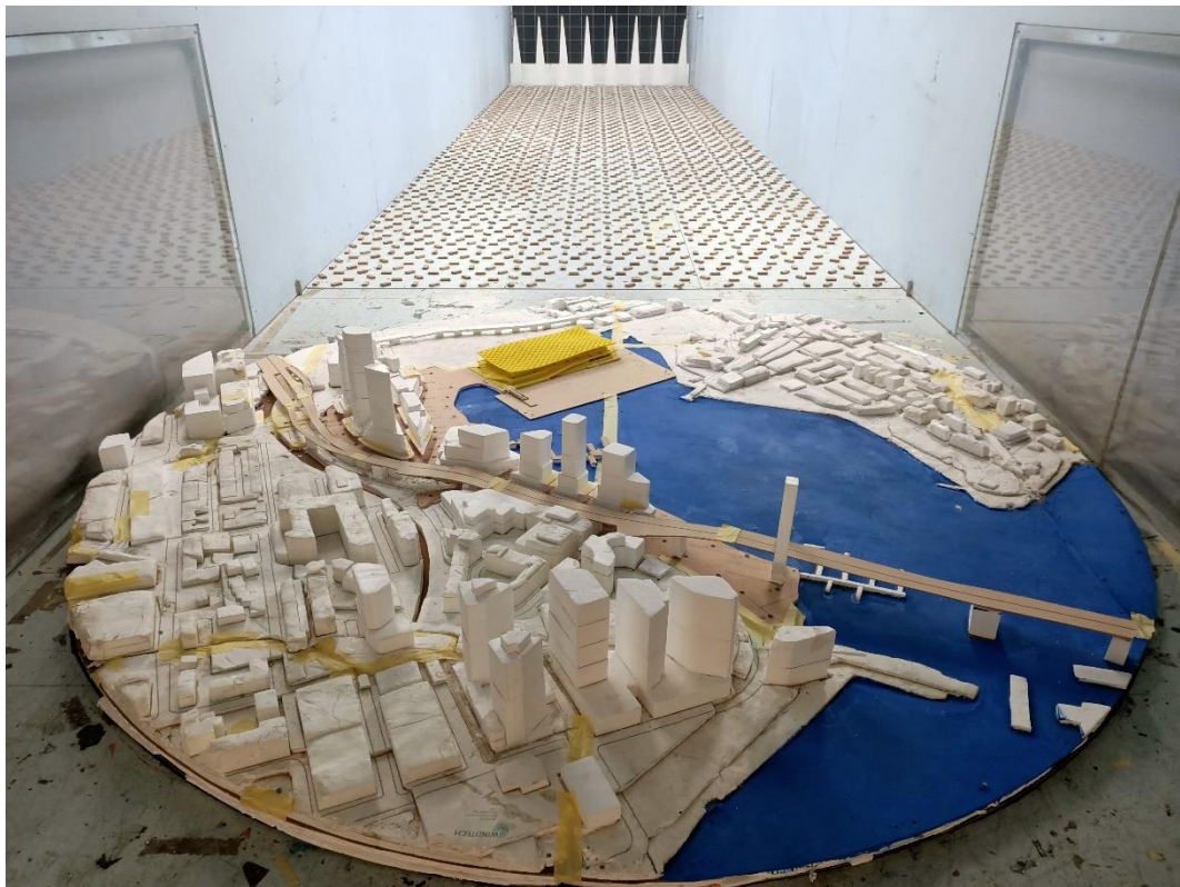
Figure 1c: Photograph of the Proposed Wind Tunnel Model (view from the north)
