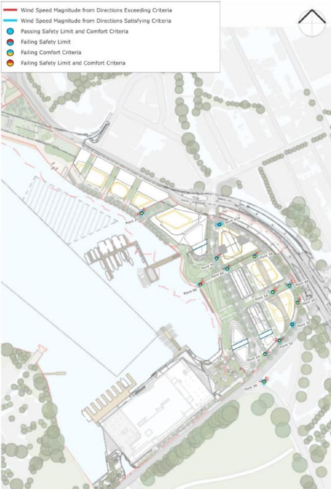
**Figure 69:** Wind tunnel results with treatments added
