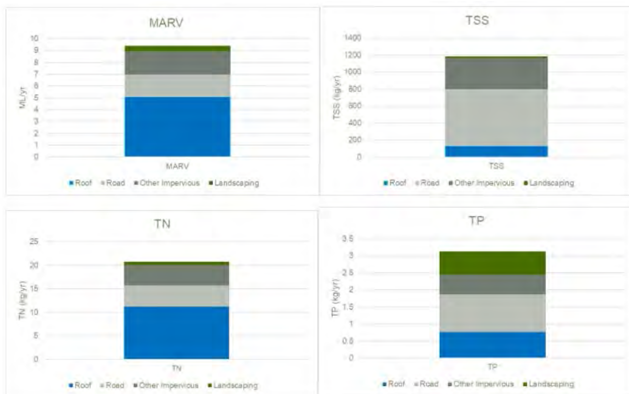
Figure 2-15 – Relative flow and pollutant generation on difference surfaces on industrial lot
