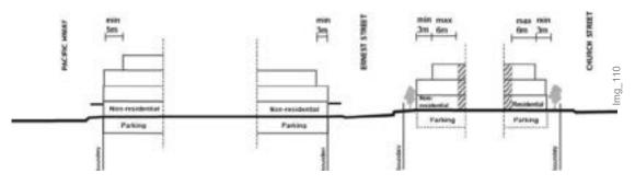
Figure 17 - Block G Section G-G
