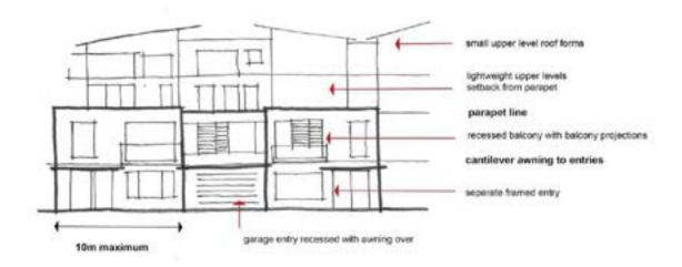
Figure 22 - Street elevation - Type E Building
