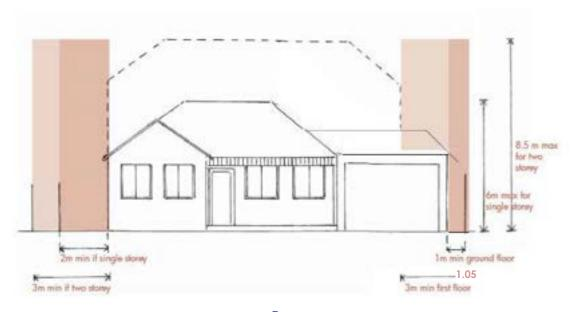
Figure 7 - Side and Rear Setbacks and Height
