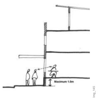
Figure 6 - Level change between footpath and ground floor level
