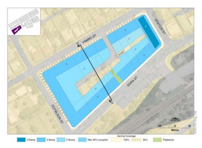
Figure 13 - Block C Control Plan
