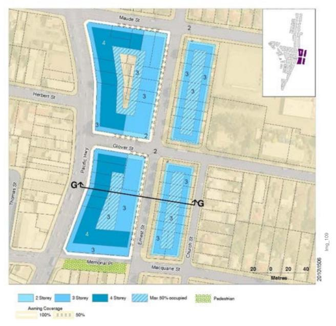
Figure 16 - Block G Control Plan
