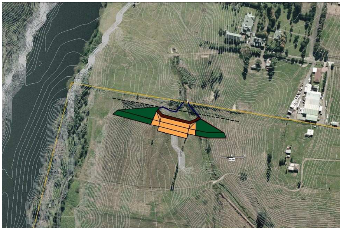
Figure 4.4 Layout of the proposed Hunts Gully Weir, option 1. (Source: Cardno Lawson Treloar, 2010)
