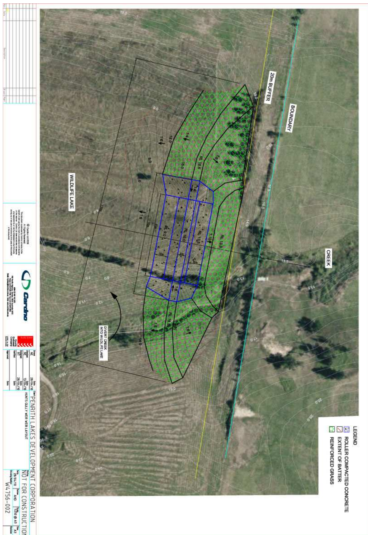
Figure 4.2 Layout of the proposed Hunts Gully Weir, option 1. (Source: Cardno Lawson Treloar, 2010)
