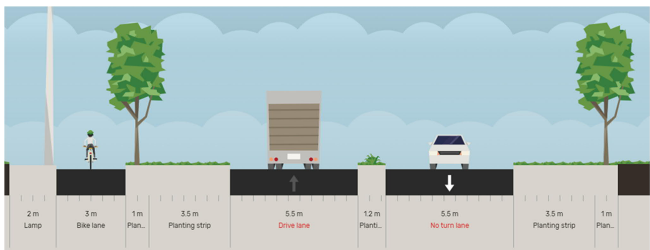
Figure 6.9 Southern Connector Road indicative cross-section
