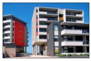
Image 6.01-19: Building separation in this residential development allows for ventilation, daylight access, view sharing and privacy
