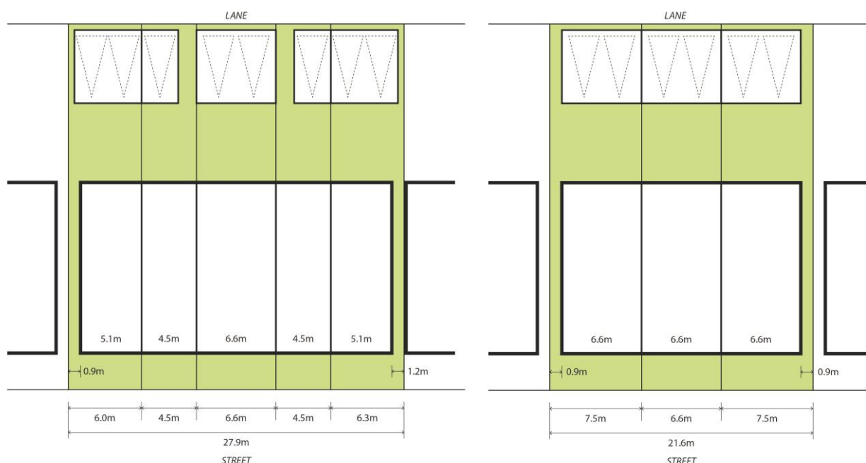
Figure 3-4. Two examples of lot subdivision for 'sets' of attached or abutting terraces
